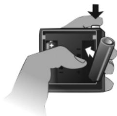
2. Press and hold the LED button while re-inserting the battery until the LED flashes red (approx. 5 seconds). The qheat RS is now reset to factory defaults.
